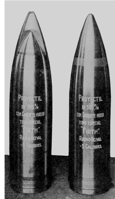
Twelve-inch AP shell with cap. (Naval Annual 1911)
